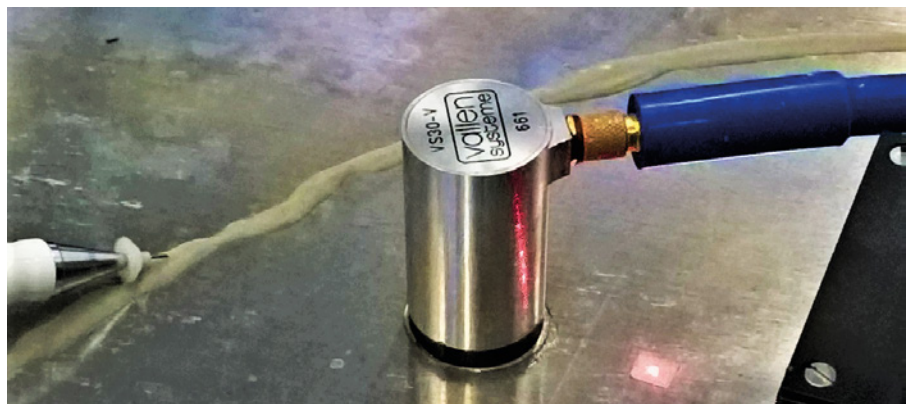
Figure 3: The three different sensors used in the experimental setup. The piezoelectric sensor, the Laser point on reflective tape and the Optical fibre glued to the AL plate. On the right, the stand for a mirror that guides the laser beam of the LDV on the plate is seen.
