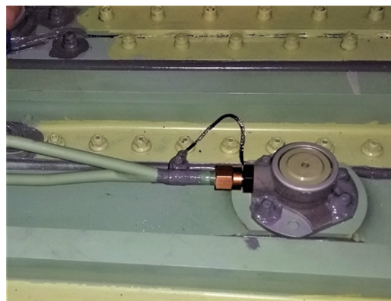
Figure 1: Left: Fuel pumps 1 and 2 with suction pipes (silver, facing towards viewer) which end at the lowest point of the wing. Right: Drain valve and suction pipe inside an AIRBUS A330 wing tank. The suction pipe connects the drain valve with the lowest point of the tank.
